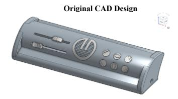
**The Odisee** is a first of its kind portable assistive scan-to-speech device for the blind and vision impaired utilizing OCR (Optical Character Recognition) software coupled with text-to-speech technology and a proprietary document organizer. The device scans mail and other documents inserted with any orientation and reads the content to the user.
